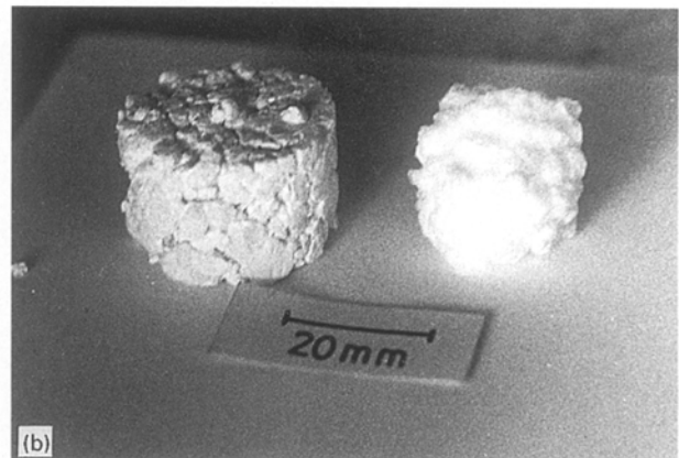
Figure 1 Expanded polystyrene (on the right) and expanded polystyrene-50 vol% alumina (on the left) mouldings at (a) 110°C and (b) 147°C.
